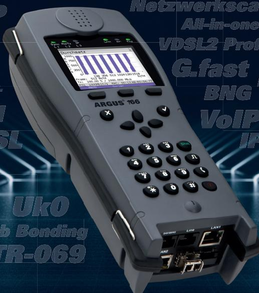
The image shows the ARGUS 166 device, a handheld testing instrument. It features a color LCD screen displaying a bar chart with the word 'Durchsatz' (Throughput) at the top. Below the screen is a numeric keypad and several function buttons. At the bottom, there are ports for SHDSL, Line, LAN1, LAN2, and a USB port.
